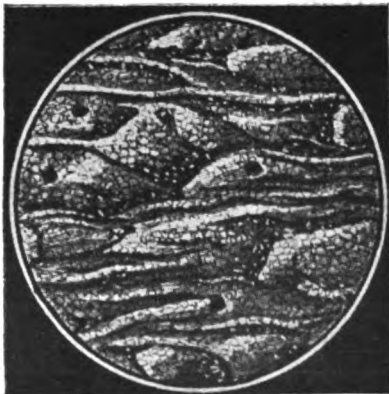
Fig. 1—Magnified surface of rough cast manganese bronze showing the semi-crystalline structure. Magnified 48 diameters
